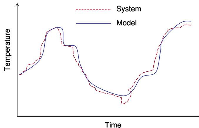
To identify a black box system a random signal (called pseudo Random Signal or PRS) input is used. This input excites the system. From the measurements of the input and output signal the system parameters can be identified and the system model can be built.
