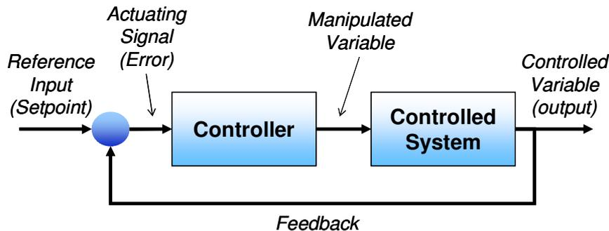
*Basic elements of a feedback control system*
