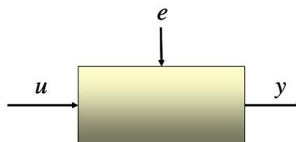
*Input Signals  $u$ , Output Signals  $y$ , and Disturbances  $e$*
