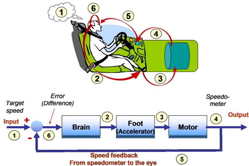
The main performance measure for a control system relates to rate of error reduction. Usually, performance is quoted in terms of the highest frequency that the control system can follow, when required to do so. All control loops tend to become unstable as higher and higher performance is sought.
